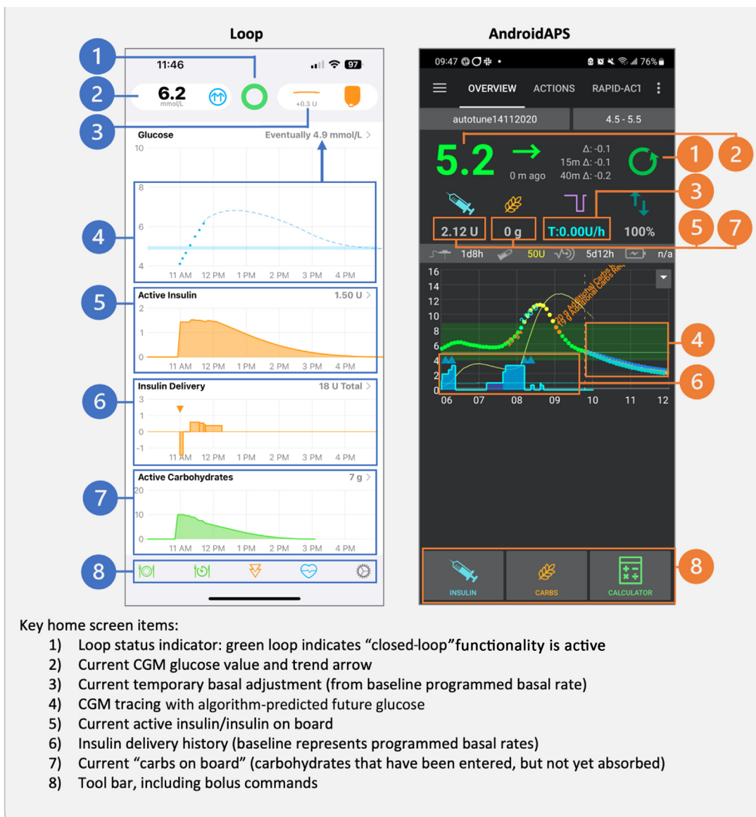
Figure 4. Sample home screen displays from do-it-yourself automated insulin delivery systems demonstrating real-time calculations. CGM, continuous glucose monitoring.
